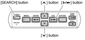
Press the [SEARCH] button while the digital video recorder is recording or stopped.
